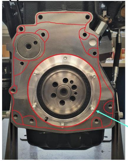
When mounting the flywheel housing, an additional surface sealant (e.g. Loctite 53-99) must be used between the engine block and the flywheel housing. In the picture on the left, the area for applying the sealant is shown in red. It is important to reproduce all the shapes shown in red as in the picture.
