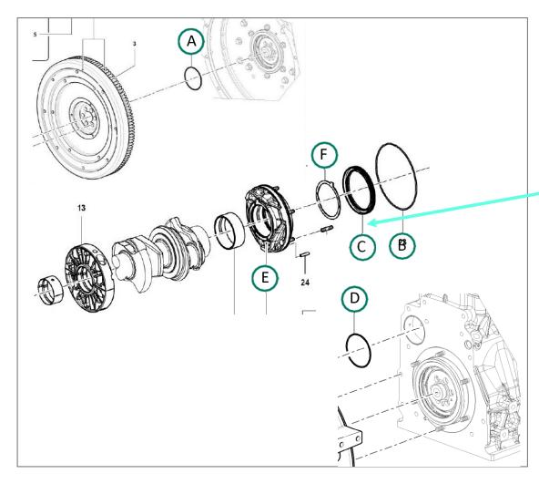
When working in the rear sealing area, always replace all seals (position A-D) as shown in the picture.
